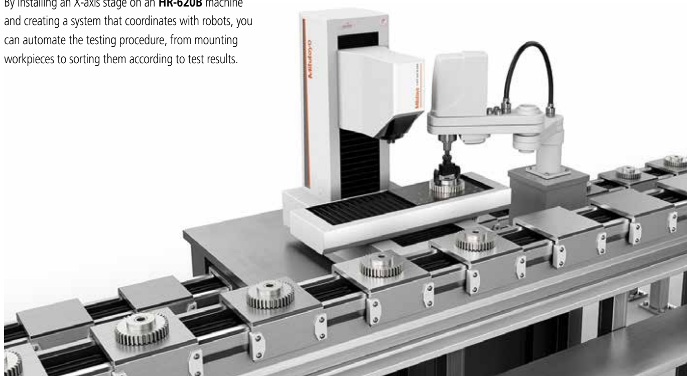
Example of hardness testing machine automation on a production line
